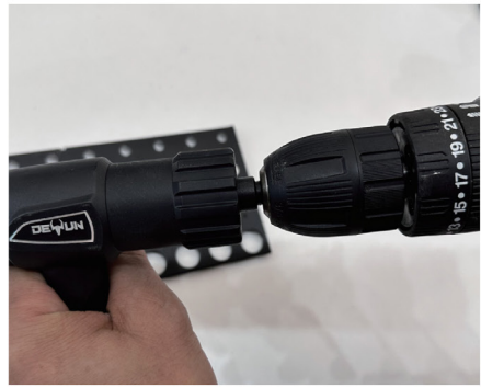
2. Open the drill chuck and insert the adapter
