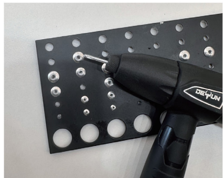
6. Turn the electric drill to reversal function, withdrawing the rivet
