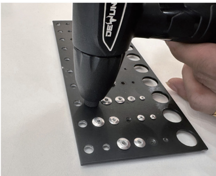
5. Turn the electric drill to corotation function, align the hole and put the rivet
